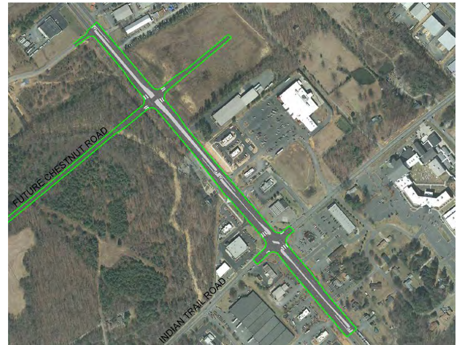
▲ Fig. 6.3 Coordinated Superstreet and Michigan Left intersections at Chestnut Parkway and Indian Trail Road
