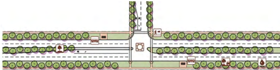
▲ Fig. 5.15 Collector Signalized Intersection
