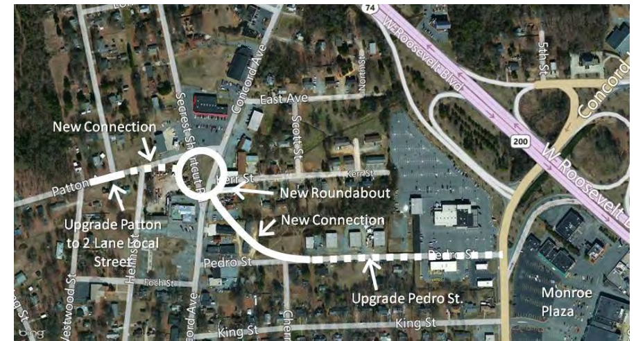
▲ Fig. 7.7 Patton Avenue to Skyway Drive Parallel Road
