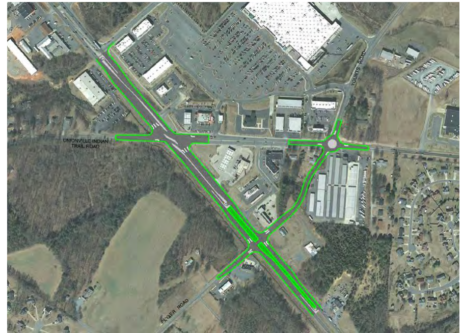
▲ Fig. 6.5 Coordinated Superstreet and Michigan Left intersections at Unionville-Indian Trail Road and Plyler Road
