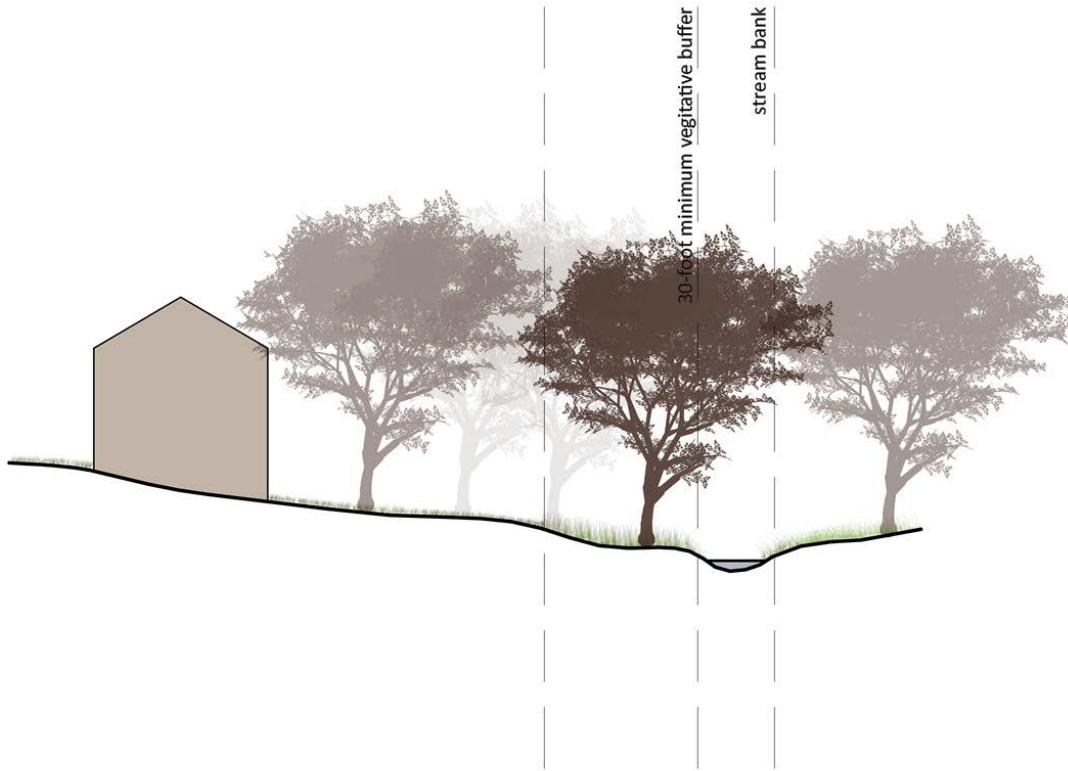
Figure 15-2: Water Supply Overlay Riparian (Vegetative) Buffer
