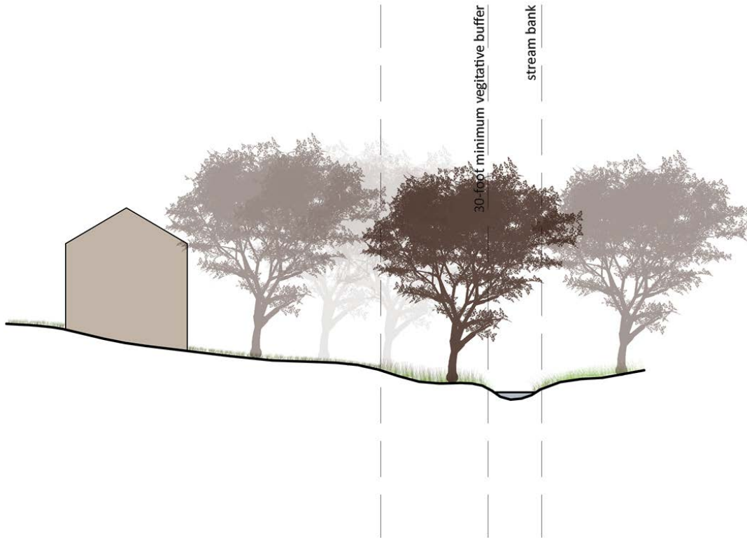
Figure 15-2: Water Supply Overlay Riparian (Vegetative) Buffer
