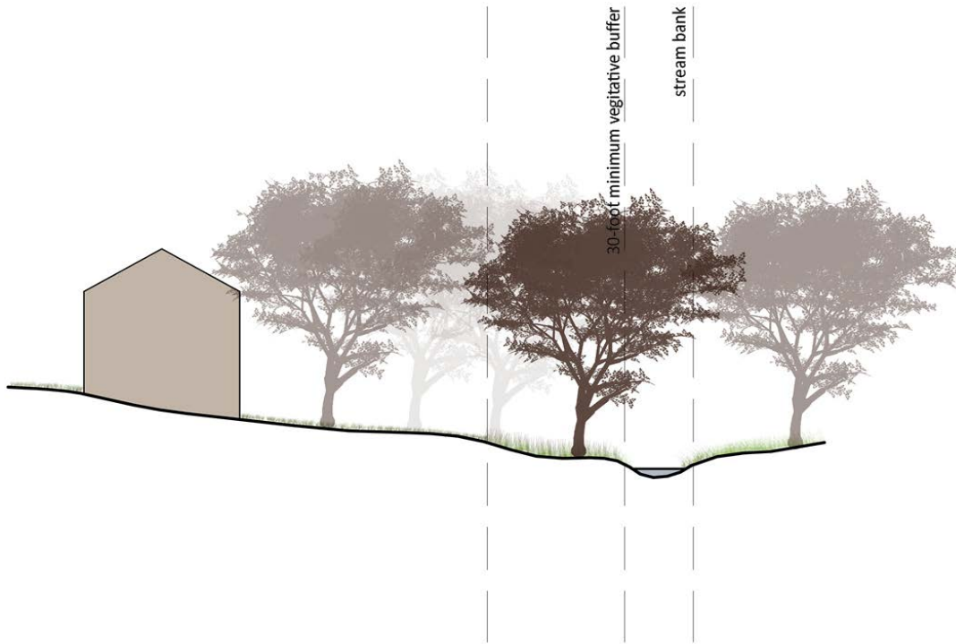
Figure 15-2: Water Supply Overlay Riparian (Vegetative) Buffer
