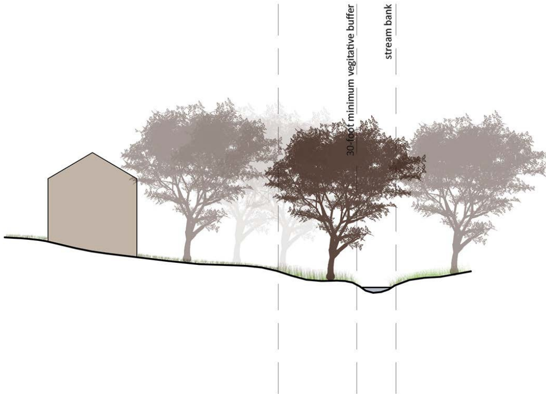
Figure 15-2: Water Supply Overlay Riparian (Vegetative) Buffer
